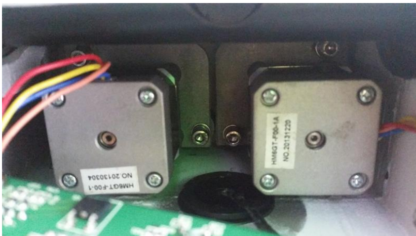
Figure 4 – Undo the two cap head bolts on each motor mounting bracket
