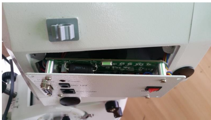
Figure 2 – Ease off the front plate
