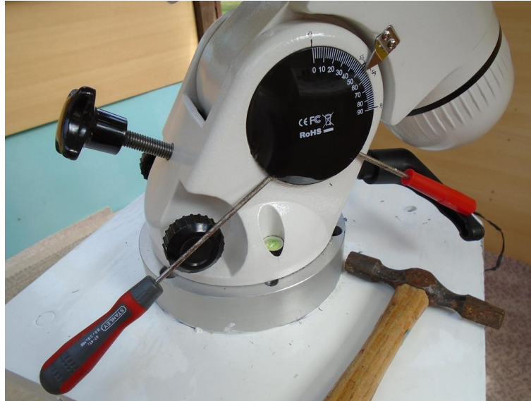
Figure 15 – Ease off the glued on covers
