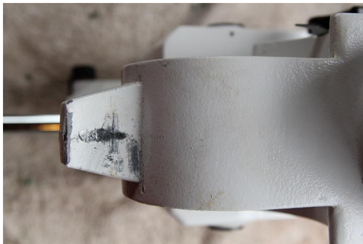
Figure 18 – Cast Tab used for antagonistic altitude adjustments
