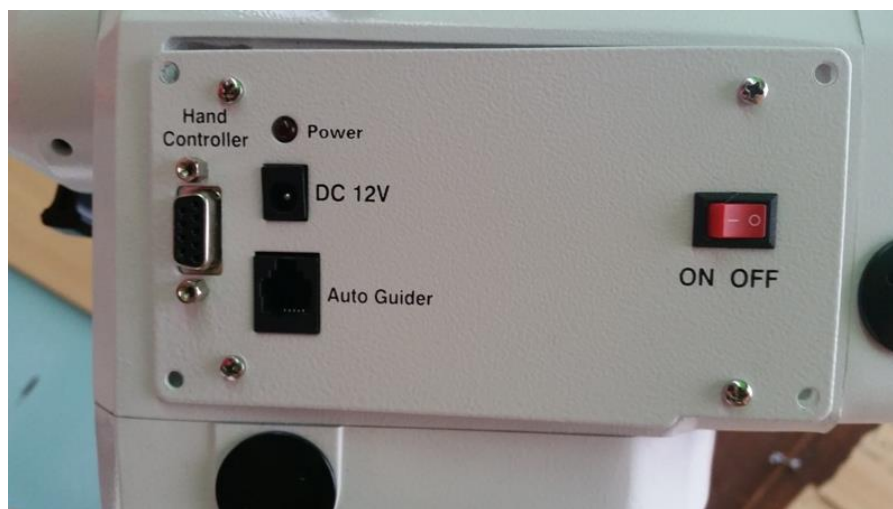
Figure 1 – Remove the four front plate corner screws
