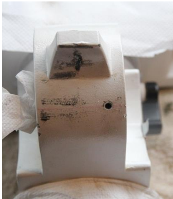
Figure 22 – Drill four holes in the mount (first one shown)
