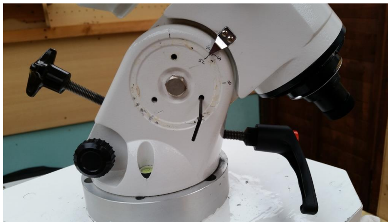
Figure 16 – EQ6 central bolt and three grub screws revealed
