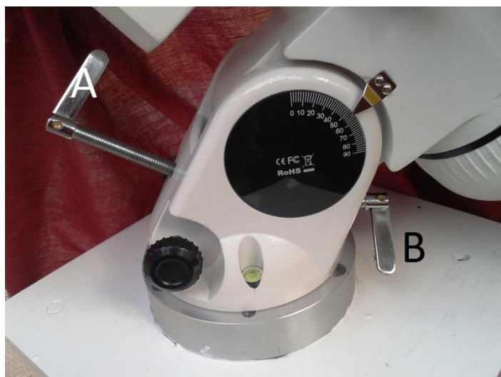
Figure 13 – Standard Altitude Adjustment bolts (set for 52 degrees)
