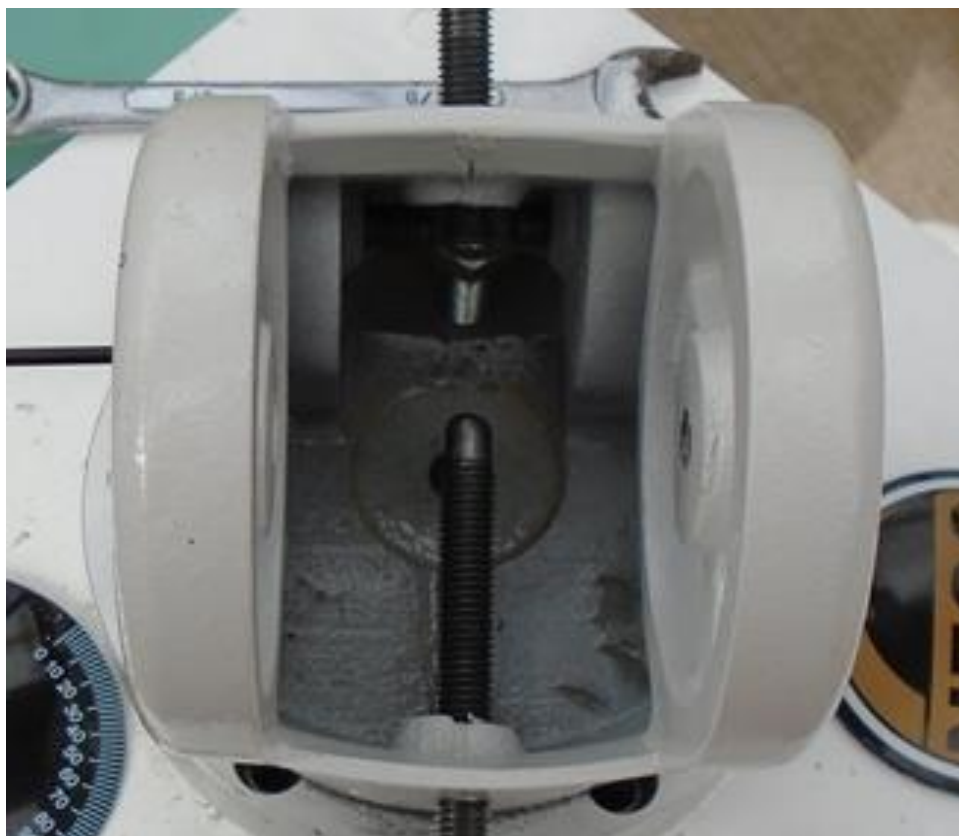
Figure 20 – Showing just how far the Altitude bolt has to be wound in for some latitudes
