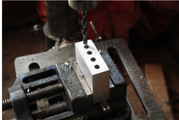
Figure 21 – Four clearance holes for 5mm cap head bolts
