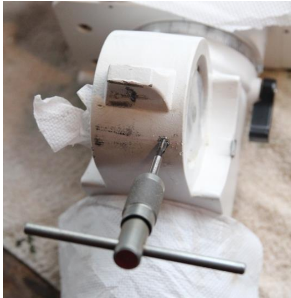
Figure 23 – Tap holes to 5mm (first one shown)
