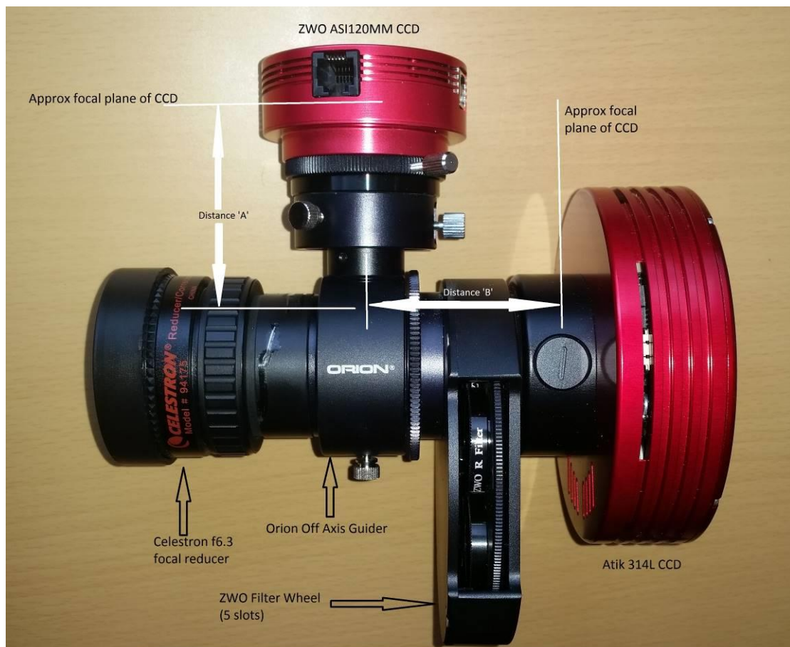
Figure 2 – Imaging setup spacing considerations
