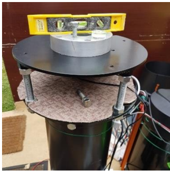
Figure 7 - Pier and mounting plate
