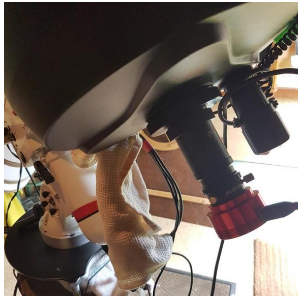
Figure 1 - Collimation via a ZWO ASI178MM camera
