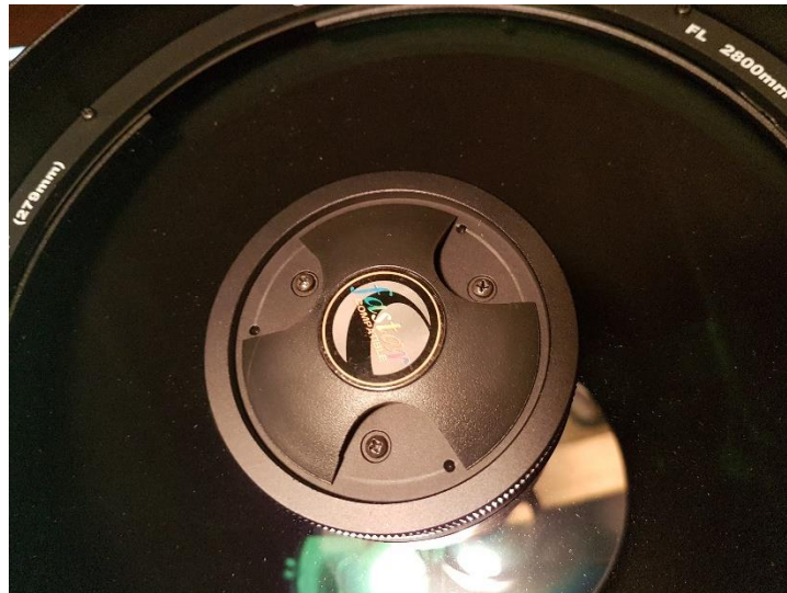
Figure 5 - Typical collimation screws (Celestron C11)
