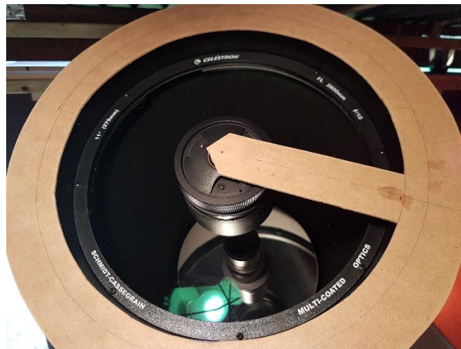
Figure 7 - Collimation aid in place
