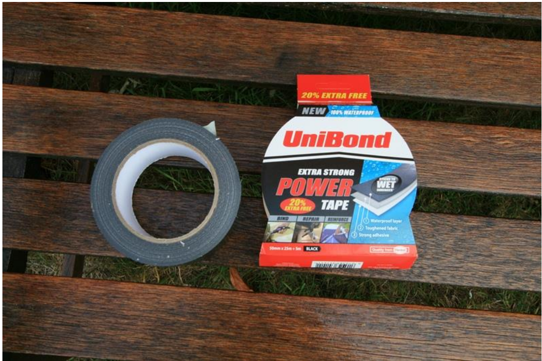
Figure 37 – Tape used to join the roof ridge sections
