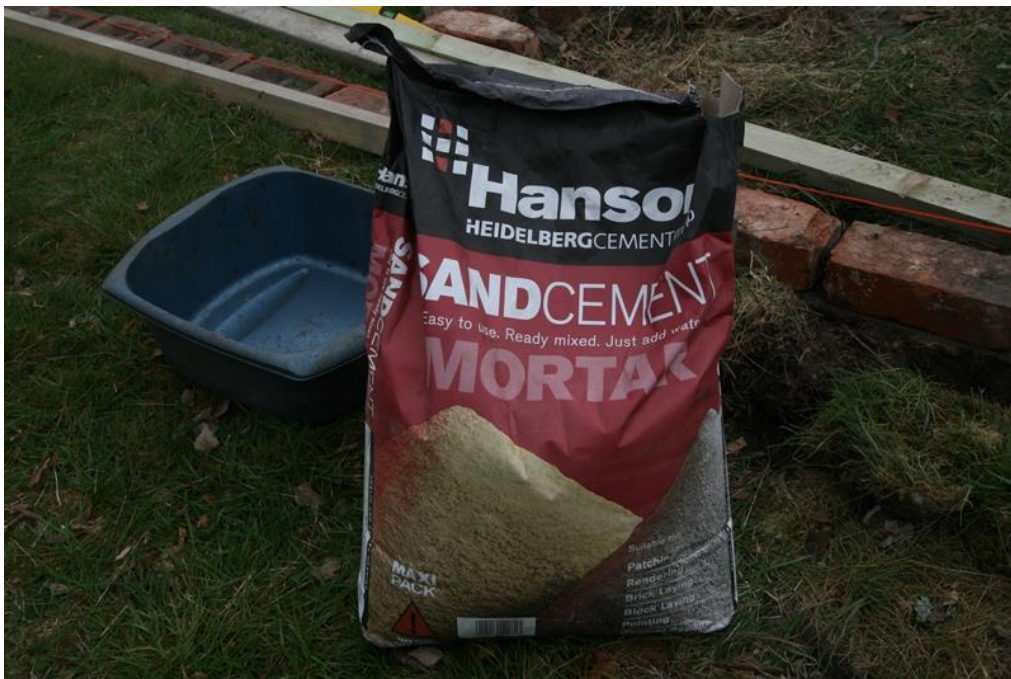
Figure 12 – Mortar for the brick laying – just add water
