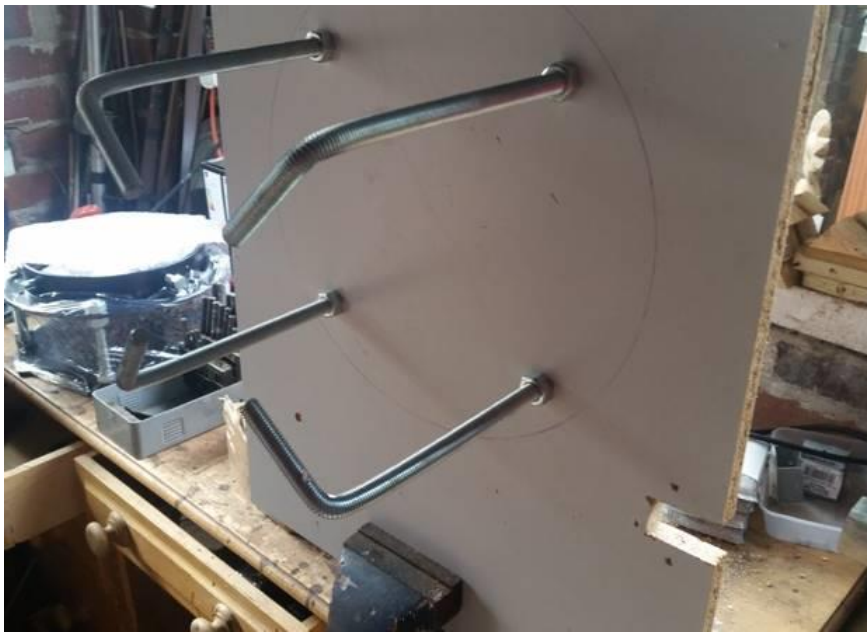
Figure 41 – Pier bolts attached to board
